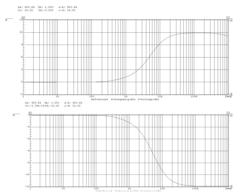
The last step is feeding the output of each of the four channels into a 4 input summing op-amp. The AC analysis was taken when the 1k source is all the way on and the others off, showing that each channel has roughly 12dB of gain. The Transient analysis shows what the waveform will look like when all of the sources are mixed together.
