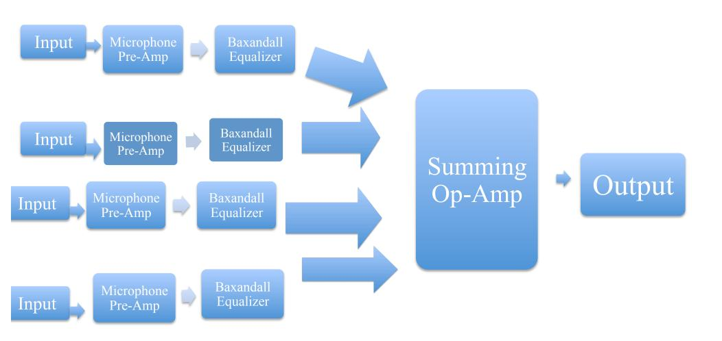
The first part of the mixing board is the microphone pre-amp. The input at V1, V2, and Ground would be the input from an XLR cable. The pre-amp has a flat frequency response between 20Hz and 20kHz and roughly 52dB of gain.
