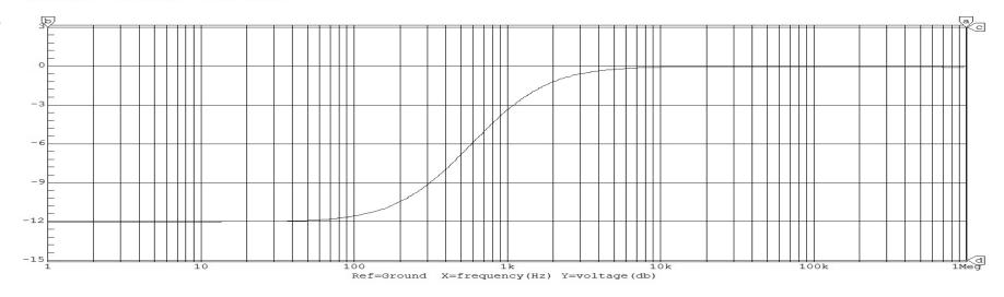
These next two AC analyses are taken when the low frequency potentiometer is at 50% and the high frequency potentiometer is at .0001% and 99.999% respectively. The .0001% graph curves back down around 1Meg, but it will not really matter because our hearing range does not go up that high.
