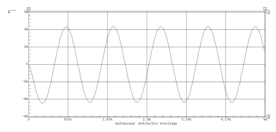
The first two AC analyses are taken when the high frequency potentiometer is at 50% and the low frequency potentiometer is at .0001% and 99.999% respectively.
